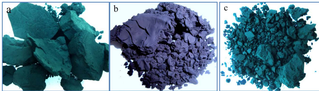
Figure 1. Photos of nonfriable and hard agglomerated powder of (a) PANI:Cl, (b) PANI-base. (c) As-dried friable and nonagglomerated PANI:p-TSA powder. [Color figure can be viewed in the online issue, which is available at wileyonlinelibrary.com .]
